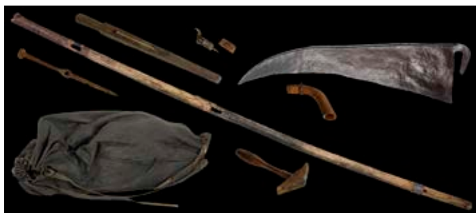
Fig. 22. Hannekemaaiers on board OB 71. Scythe in loose parts and devices, mainly for sharpening the blade of the scythe: chine, snaith, snaith crutch, peening hammer, peening anvil, grip, strickle and kit-bag (photo Penders, RCE, composition Boersma, GIA).
