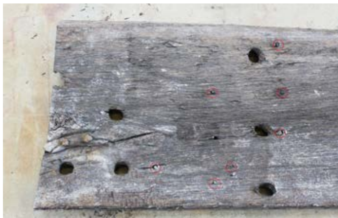
Fig. 31. Spike-plugs (spijkerpennen) in one of the bottom planks of OE 34 (photo IFMAF).
